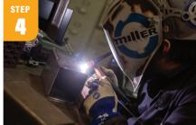
Now it's time for the silicon bronze rod. Do any welding you're going to do first, because you can braze SiB over ss, but it's not fun trying to weld with mild or stainless filler metal over the silicon bronze. TIG braze all the vertical seams. I'm using DC on these joints, but you can also TIG braze using AC. Dealer's choice.
