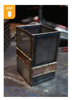
Make sure it doesn't leak! Add some water while keeping the outside dry. Set it on a dry surface, and let it sit while inspecting all the edges and the corners. If it leaks, you'll need to grind out that spot and weld/braze it again.
