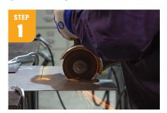
Measure and cut the stainless steel and mild steel plates to size. In this case, the dimensions are 4"x4" for the base and 4"x7" for the sides. Then cut two pieces of copper 1" wide and over 8" long. Leave a little extra length on the copper for fit-up. Once you've laid out the cut lines, use your cutting wheel, saw or plasma cutter to cut the steel. Clean up the edges with a flap disc.
