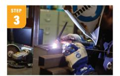
Clean the edges with a wire wheel or brush. Weld the bottom four edges using the stainless filler. Take care to wrap the corners; those are the most problematic spots for leaks.
