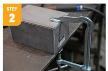
Square up the sides in pairs. Use a 90° block of some sort with a clamp to hold them in place, then tack them together. Put the mild steel sides opposing each other, then fit the stainless steel pieces on either side of them. Make sure the bottom and the sides are all tacked together, and keep fit-up in mind for a nice corner to weld.
