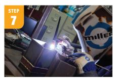
To finish off the welding/brazing, run little beads around the top edges of the vase. It rounds them off, taking away any sharp corners, and it adds a little style.
