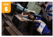
Begin laying down SiB beads on the edges of the copper to the face of the steel. Again, take your time and run short beads; you'll have to continue to hammer and clamp the copper to keep it flat. The characteristics of the materials are very different, so be patient. If you leave too much of a gap under the copper, you'll blow through it. Keep it tight to the steel as you move around with the filler and the TIG torch, leaving no edge untouched.
